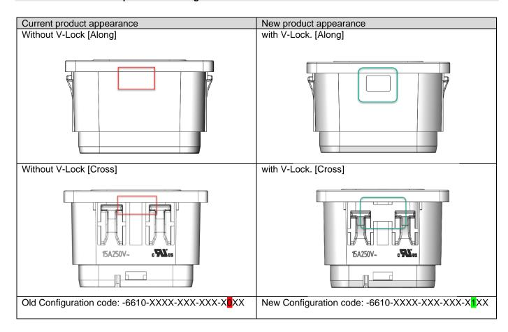
Change socket design from without V-Lock notch to with V-Lock notch.
